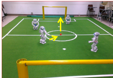
Fig. 1. The initial condition is that the striker has a good location estimate and plans to kick the ball toward the opponent's goal.
