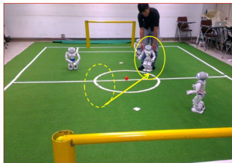
Fig. 2. The striker is manually placed to the symmetric pose and the striker will have an incorrect location estimate. It is very likely that the robot will incorrectly kick the ball toward its own goal.
