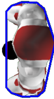
Figure 9: Examples for “Ball Holding”. The black circle is the ball and the blue polygon visualizes the convex hull of the robot’s projection onto the ground. Situation a) is legal, whereas b) violates the rule.
