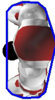
Figure 10: Examples for “Ball Holding”. The black circle is the ball, the blue polygon visualizes the convex hull of the robot’s projection onto the ground and the red area shows the occupied portion of the ball. Situations a) is legal, whereas b) violates the rule.
