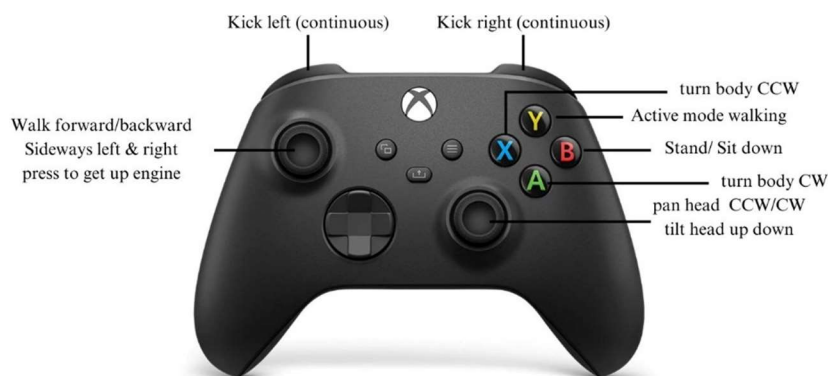
Figure 2: Xbox Controller Button Mapping in Linux
