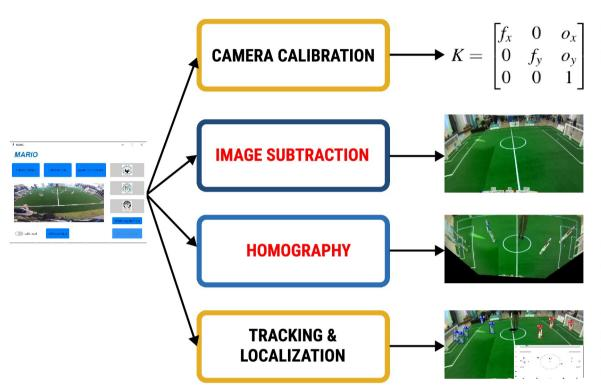
Among a set of intrinsic parameters of the camera, those with a minimum reprojection error have been chosen.
