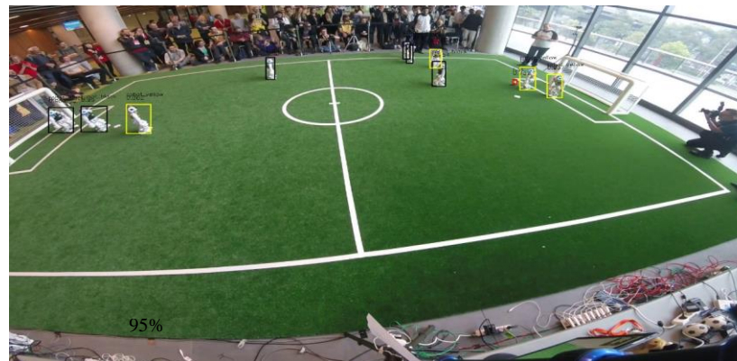
Fig. 2: Output of the Yolo5. network. The labelling for the subsequent training phasse was done semi-automatically by means of tools and manual correction.
