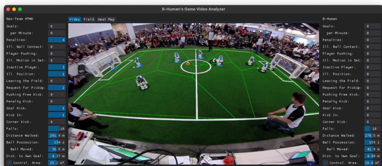
Application showing the video of a half not in the training set with positions of ball and players (big circle indicates fallen robot). The statistics determined from the GameController log and from the video are shown next to the video.
