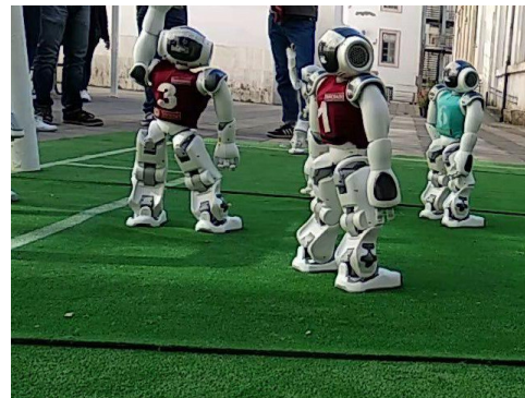
Figure 1: An example of the SPL scenario used to demonstrate the hand-gesture communication. The kicker and the receiver have the raised hand to perform the visual handshake.
