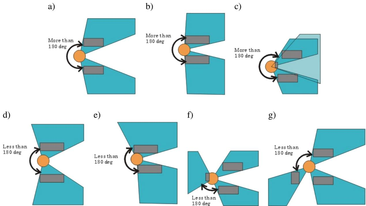
Figure 10: Examples for “Ball Holding”. The orange circle is the ball, the grey boxes are parts of the robot, and the blue area visualizes the ranges occupied by the robot. Situations a), b) and c) are legal, whereas d), e), f) and g) violate the rule.
