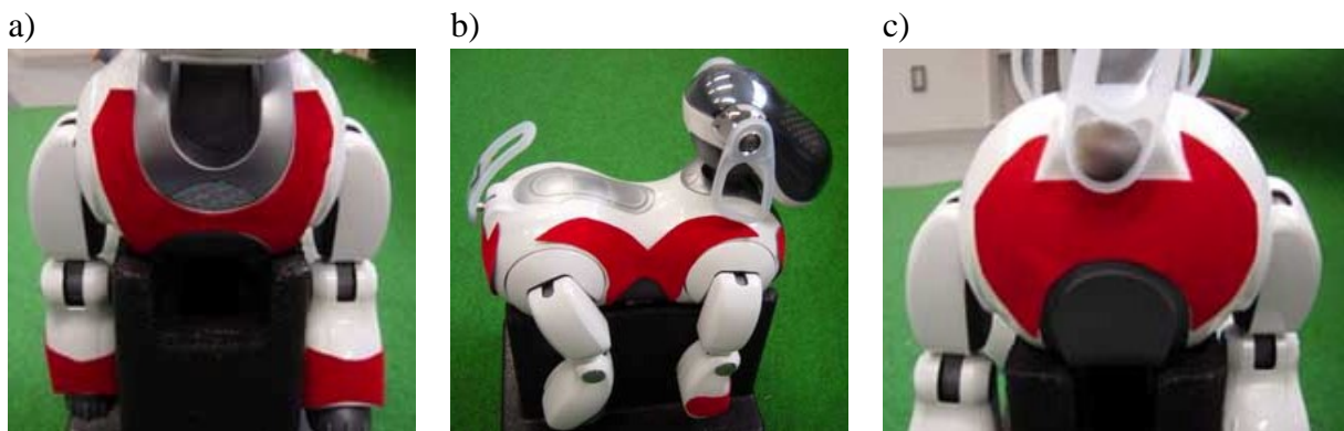
Figure 6: ERS-7 team markers. a) Front view. b) Side view. b) Back view.
