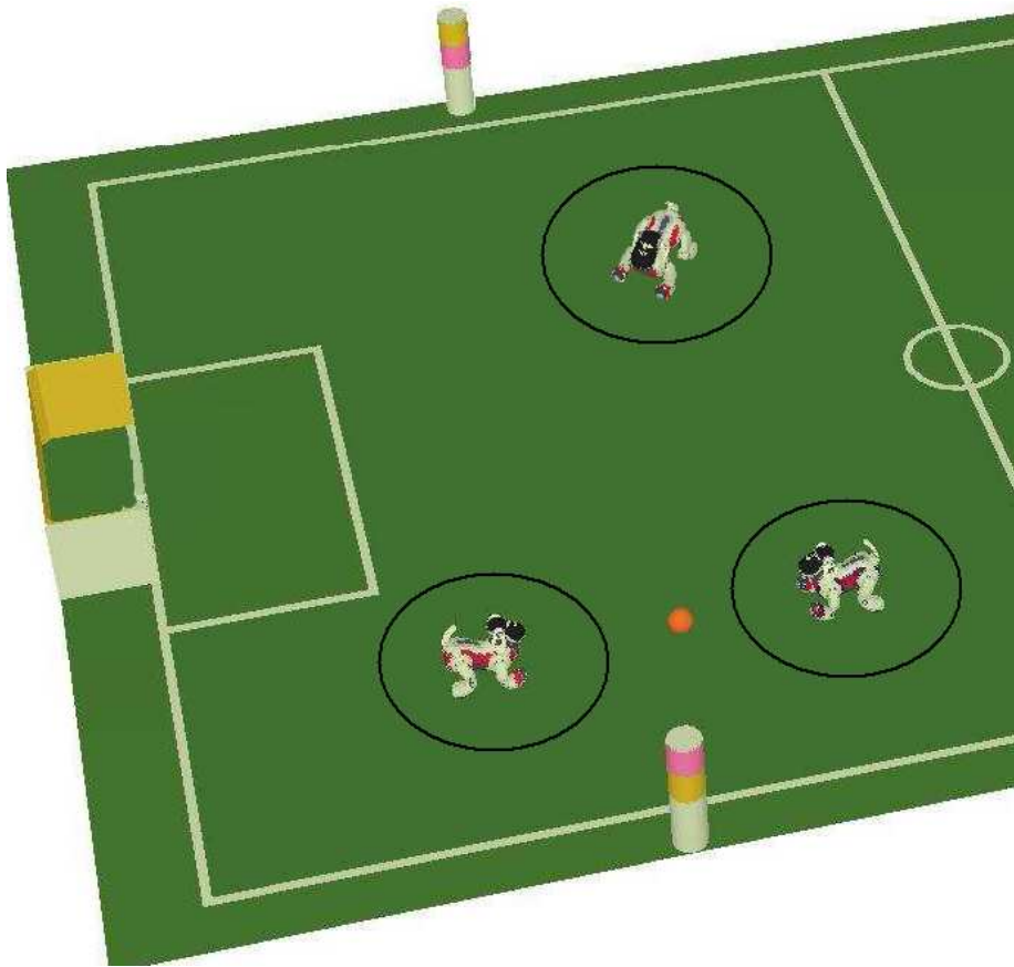
Figure 1: An example placement of the robots for the passing challenge. The circles will be drawn on the field but will not be visible to the robot.
